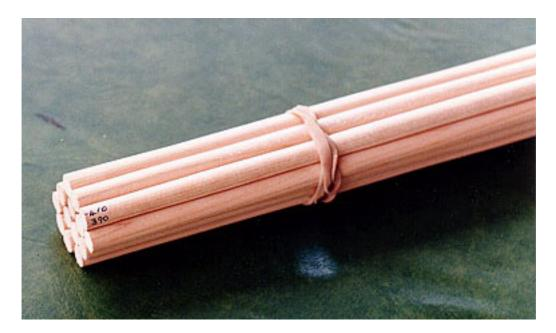
Raw Shafts, with grain and spine weight marked. Note the rubber bands keeping shafts tightly secured: This helps to keep them straight over time.
