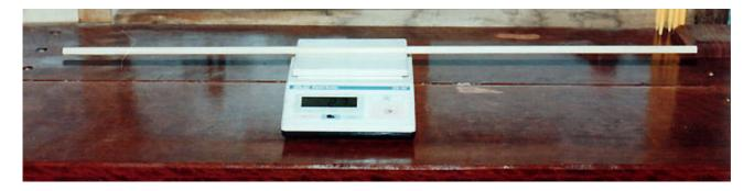
Weighing the shaft on a grain scale.
