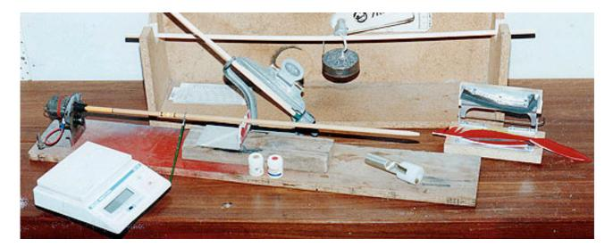
Clockwise from bottom left: Grain Scale, Cresting Jig, Fletching Jig, Spine Tester (at rear), Feather Chopper, Tapering Tool.
