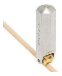
**Tech Tip:** You can buy expensive Arrow Straightening Tools as pictured or make your own from a slotted piece of Timber with a Steel Roller bolted in place, a piece of Dowell and a Cup Hook or a simply use the Shaft of a Screwdriver to gently stroke the Bend. Be careful, you are relying on Wood Fibres being compressed at the Bend Site to keep the Arrow Shaft straight. Take your time, be gentle, and don't crush the Timber Fibres.
